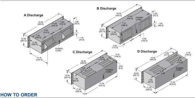
Specify model number, adding discharge suffix A, B, C or D. Example: KP1051A Rev. A. For 230 VAC operation, add a 2 after the K. Example: K2P1051A Rev. A. Dimensions, inches [mm], are for reference only and subject to change.
