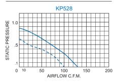
Airflow vs. static pressure curves are shown for 60 Hz (solid line) and 50 Hz (broken line) inputs. Static pressure is in inches of water.
