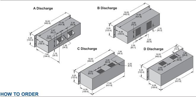
Specify model number, adding discharge suffix A, B, C or D. Example: KP528A. For 230 VAC operation, add a 2 after the K. Example: K2P528A.
