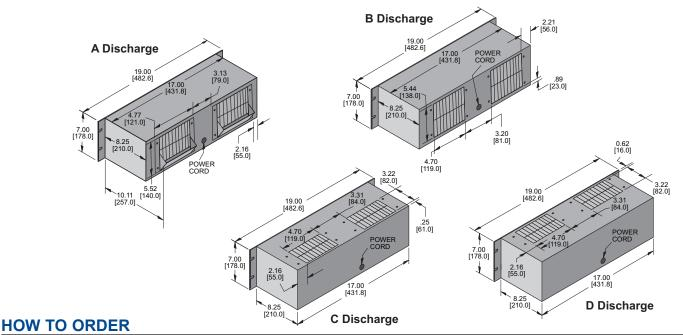
Specify model number, adding discharge suffix A, B, C or D. Example: KP701A. For 230 VAC operation, add a 2 after the K. Example: K2P701A.
