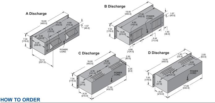
Specify model number, adding discharge suffix A, B, C or D. Example: KP729A. For 230 VAC operation, add a 2 after the K. Example: K2P729A.
