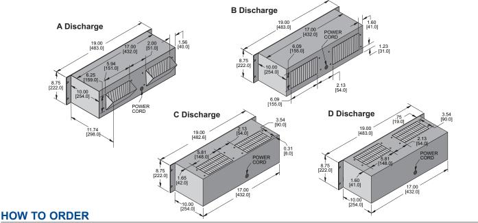
Specify model number, adding discharge suffix A, B, C or D. Example: KP877A. Unvailable in 230 VAC.
