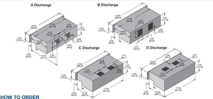
Specify model number, adding discharge suffix A, B, C or D. Example: KPL701A. For 230 VAC operation, add a 2 after the K. Example: K2PL701A. kpl701.qxd (8/1/23) (CDR: 20498)
