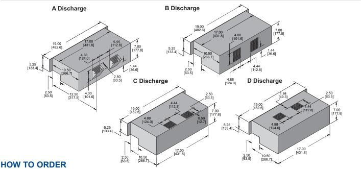
Specify model number, adding discharge suffix A, B, C or D. Example: KPL729A. For 230 VAC operation, add a 2 after the K. Example: K2PL729A. kpl729.qxd (8/1/23) (CDR: 20498)
