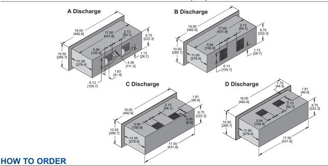
Specify model number, adding discharge suffix A, B, C or D. Example: KPR877A. Unavailable in 230 VAC.
