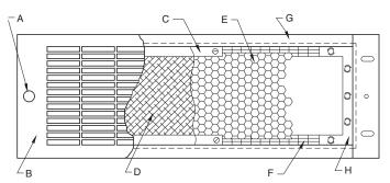
**EMI-SHIELDED FILTER-GRILLE ASSEMBLIES:** (A) Captive Thumbnut, (B) Grille, (C) Plated Steel Retainer Frame, (D) Aluminum Filter, (E) Honeycomb, (F) EMI Gasket (Plated knitted wire mesh), (G) EMI Frame (Plated steel rear surface), (H) Plated steel surface.
