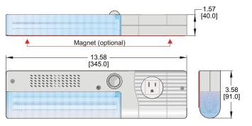
Note: A Passive Infrared (PIR) motion sensor detects the motion of the enclosure door being opened and automatically turns on the light. The sensor is factory pre-set to turn the light off 5 minutes after all motion ceases. The motion sensor does not detect movement through glass or fiberglass, thus allowing installation in enclosure with glass doors.
